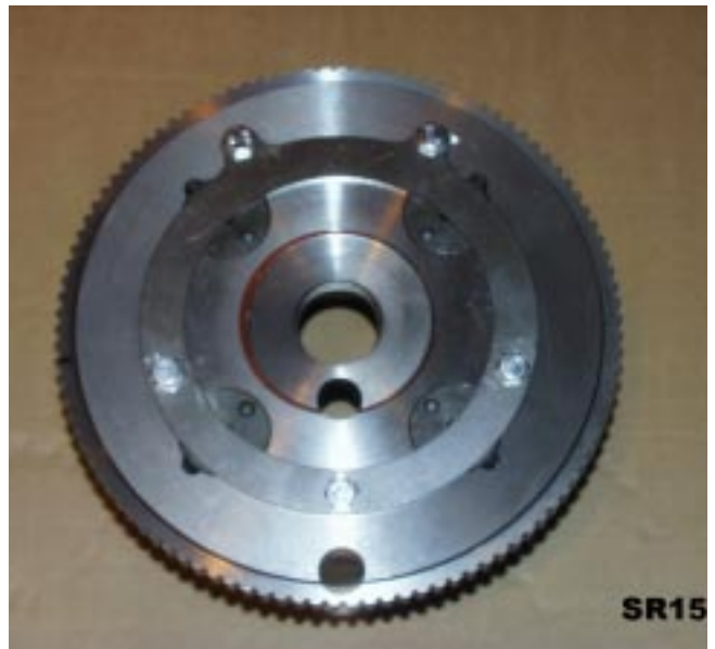
Picture 14: planetary wheel pin locking plate installed
