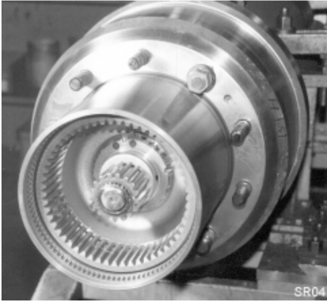
Picture 7: Planetary housing when planetary carrier is removed
