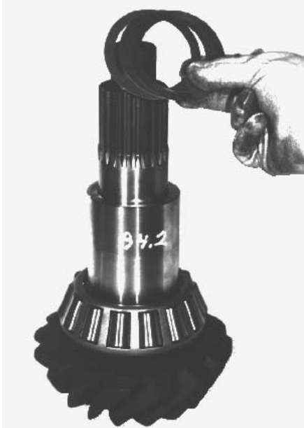
Picture 8. Pinion with inner bearing cone installed.
