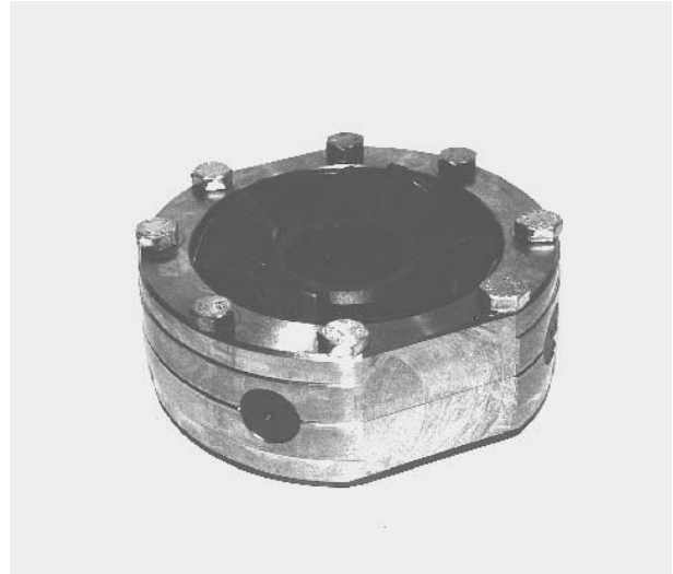
Picture 4. Inter-axle differential assembly.
