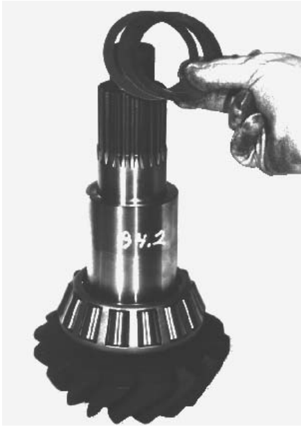
Picture 8. Pinion with inner bearing cone installed. Note installation of spacer bushing and shims
