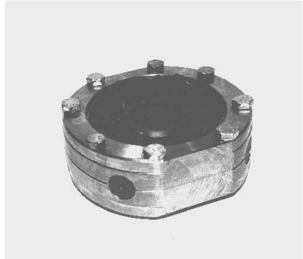
Picture 4. Inter-axle differential assembly.
